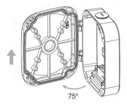
Step 2: Loosen the screws of the fix rings, put rings through the back of the box body;
