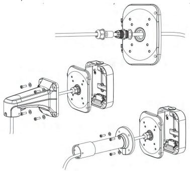
Step 8: The box supports top or bottom cable-out ways as below picture, through the top hole, or tension disc which put cables through bottom or bottom back. For tension disc, please remove it then cut an opening on the rubber plug, get cables through the opening. Please remember to plug the rubber plug whenever the holes on it are not in use;
