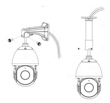
Step4: Make sure that the camera body has been correctly installed to the holder, and match the holder to the holes on the wall or ceiling, then tighten up the screws;
