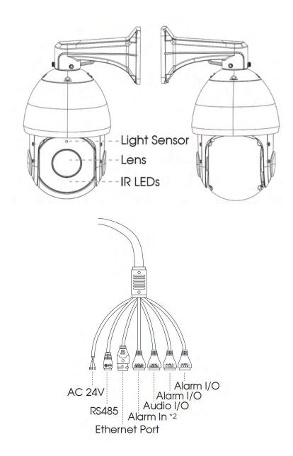
NOTE: 1) Only AC 24V is available for Speed Dome Network Camera power supply. AC 24V and PoE+ (802.3at) are available for PoE Speed Dome Network Camera power supply;
